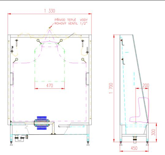
This device is used for aprons and working boots cleaning and disinfection. It is used mostly in food industry in hygiene stations. The box is equipped with hooks on which are hooked aprons. Washing is done with hot water and sprinkler head and showering brush. The device is made of stainless steel and answer to high demands for clearing and hygiene.
